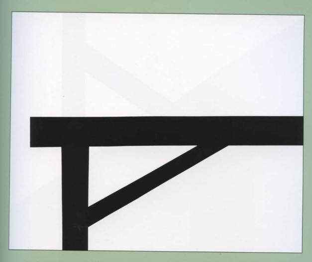
A diagonal strut holding in place a vertical stud and a horizontal beam is in tension, supporting the one, restraining the other, and tying the two securely together as a much more stable unit.
