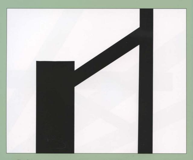
The flying buttress is an architectural device that was invented to enable the builders of Gothic cathedrals to construct walls ever higher and ever thinner, helping to give an airy, almost weightless feeling to these structures. If a roof had been built on these walls without their having additional support, they would have buckled outward from the pressure. Flying buttresses are diagonal wedges braced against thick outer walls to support the inner shell of the cathedral.
